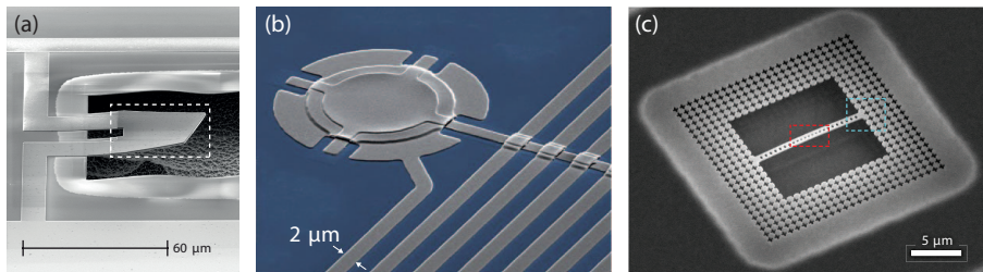
FIGURE 1.4: Geometries with which the quantum ground state of a mechanical resonator has been reached: a) A bulk dilatational resonator coupled to a superconducting phase qubit [13], b) an aluminium nanodrum in a superconducting LC electrical resonator [14], and c) a patterned silicon nanobeam, surrounded by an external phononic bandgap shield [15].
