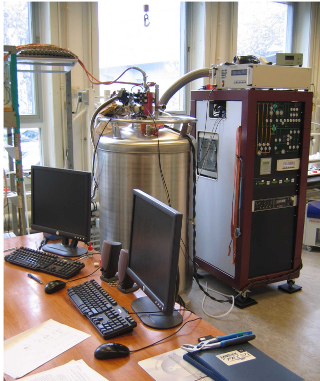
Figure 5.8: Photo of the measurement setup. On the right side sits the Gas Handling Unit. The refrigerator is situated in the middle, between the Gas Handling Unit and the matrix modules with the DACs at the left edge. All sample currents and voltages, as well as the data storage, is carried out through home-made computer software.
